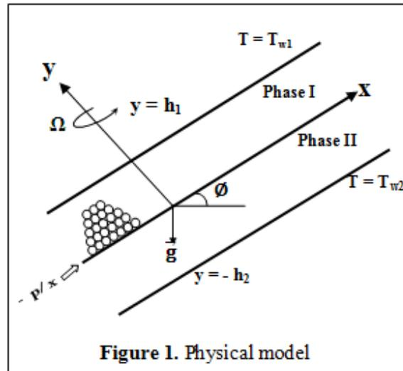
The transport properties of the two fluids are taken to be constant. Further, the flow is assumed to be steady, laminar, fully developed and driven by a constant pressure gradient ( $-\partial p/\partial x$ ). The whole system is rotated with an angular velocity  $\Omega$  about the  $y$ -axis. The governing equations of motion and energy for phase I (porous medium) and phase II (clear viscous fluid) are formulated with the above assumptions.
