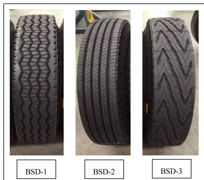
Figure 8. Tyre tread patterns of the 20.00-10 biased pneumatic retreaded truck tyres
