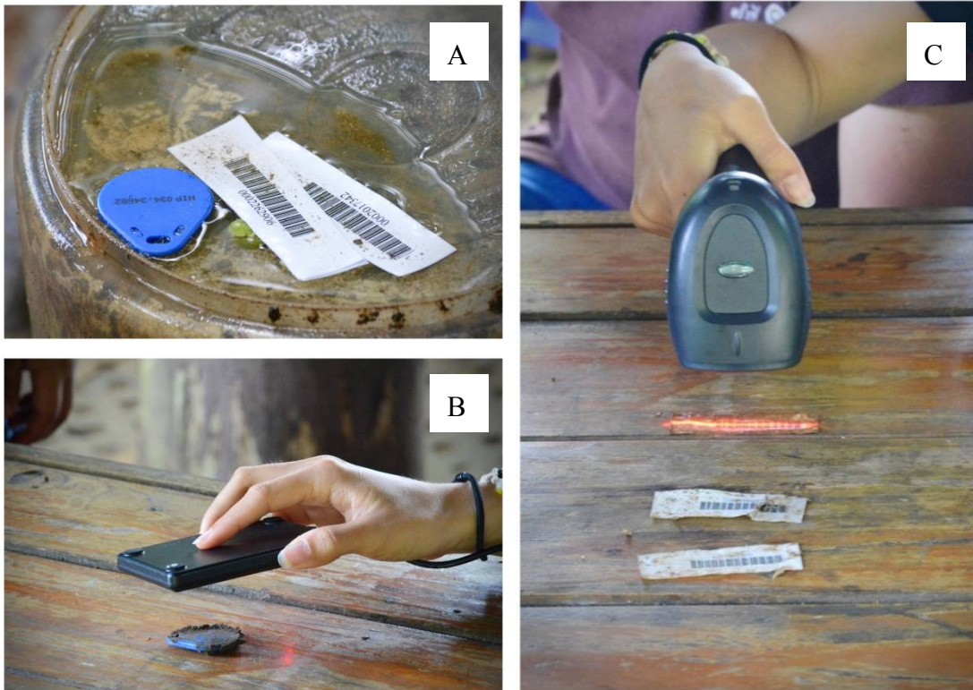
Figure 2. Readability test: (A) tags and barcodes are soaked in water before being read in order to study their moisture resistance; (B) readability testing of dirty RFID tag; (C) levels of dirtiness of barcodes assessed are heavy, moderate and light.
