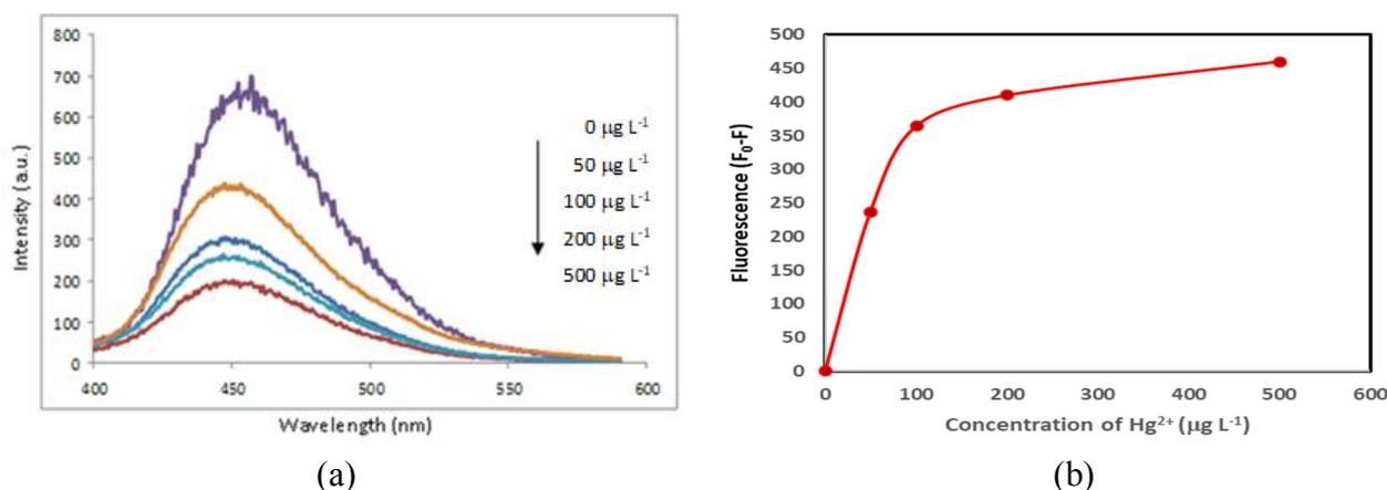
**Figure 5.** (a) Fluorescence spectra of 400 mg L<sup>-1</sup> TNK-CDs solution after addition of Hg<sup>2+</sup> at different concentrations; (b) Fluorescence/concentration graph for quenched Hg<sup>2+</sup>, showing linear portion of the curve between 0-100 mg L<sup>-1</sup>
