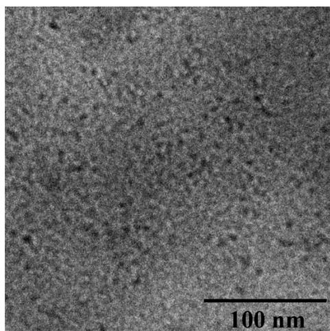
**Figure 2.** Typical TEM image of the TNK-CDs
