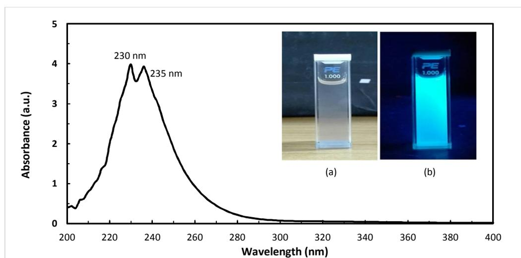
**Figure 3.** UV spectrum of purified TNK-CDs; inset shows photographs of TNK-CDs aqueous solution under (a) daylight and (b) 365-nm UV light
