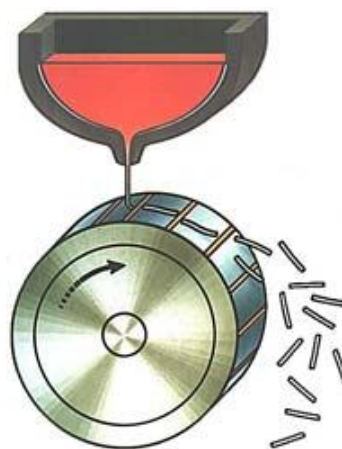
Figure 1. Production process of amorphous metallic fibre
