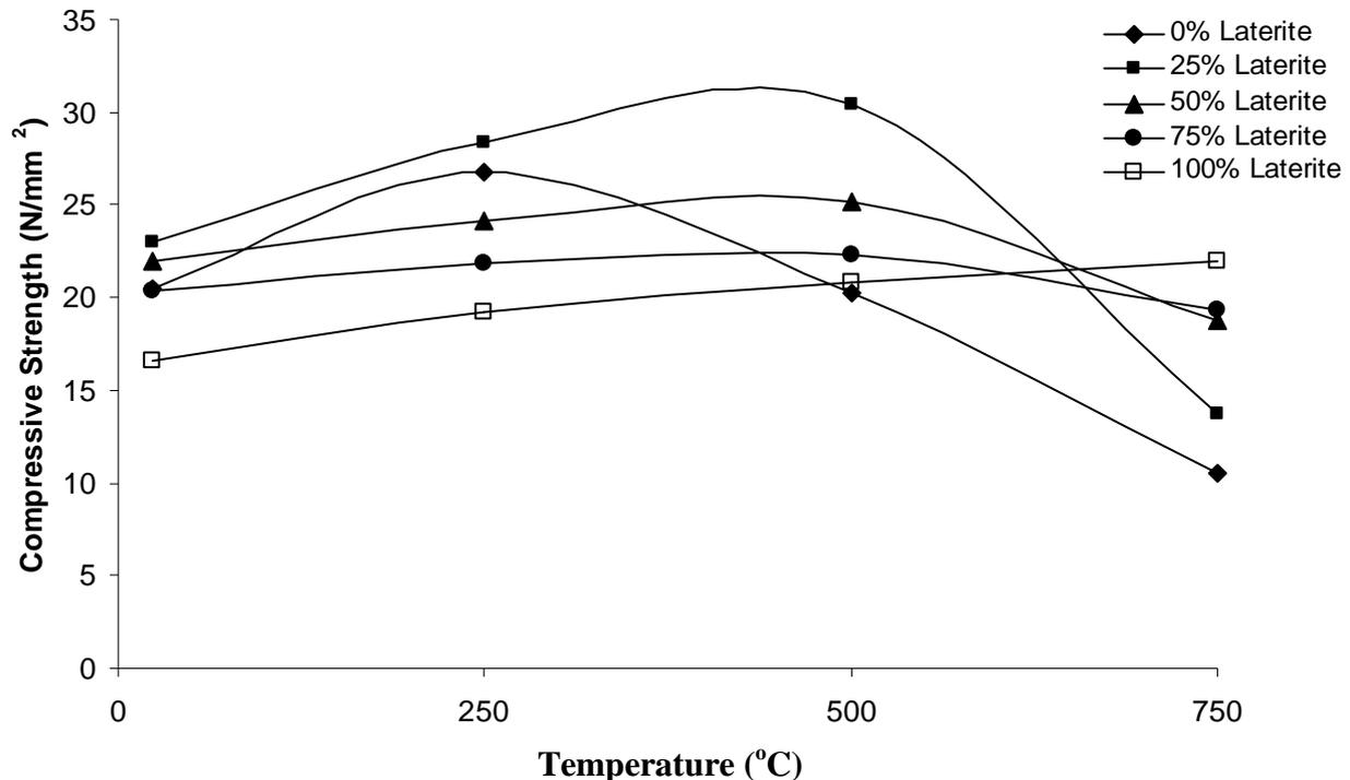
**Figure 3.** Variation of compressive strength with temperature for concrete of 28-day curing age with different levels of laterite content
