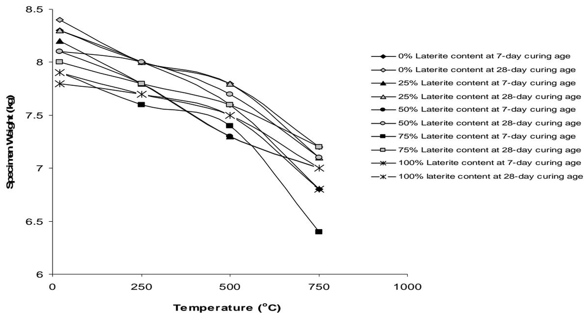
**Figure 2.** Variation of specimen weight with temperature for various values of laterite content at 7 and 28 days
