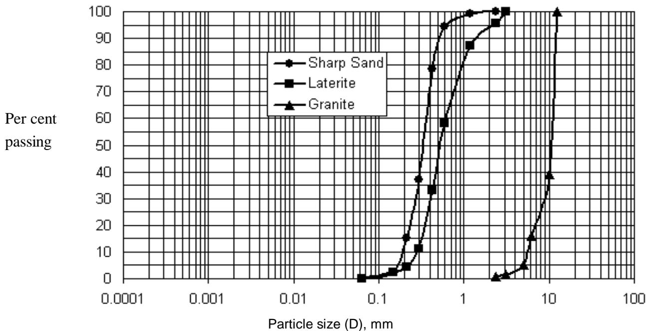
**Figure 1.** Particle size distribution of the aggregates
