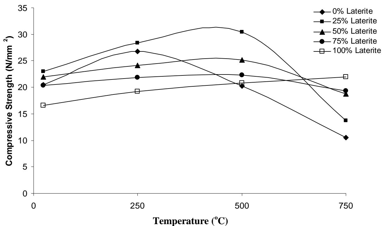
**Figure 3.** Variation of compressive strength with temperature for concrete of 28-day curing age with different levels of laterite content
