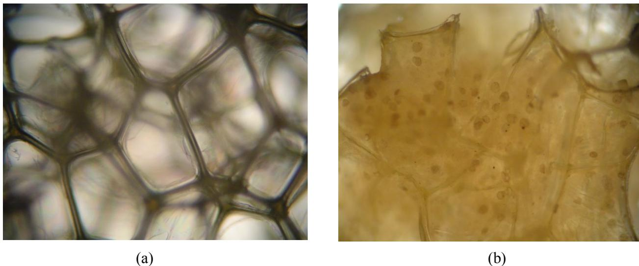
**Figure 12.** Photographs of sponge medium surface ( $\times 10$  magnification): (a) without bio-sludge, (b) with bio-sludge
