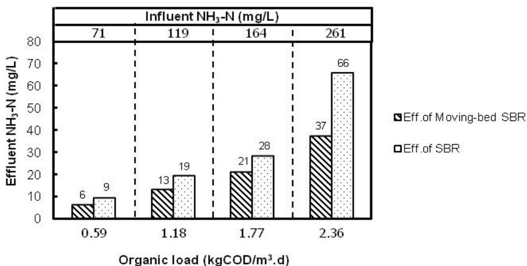
Figure 9. Variation in effluent ammonia-N with organic load
