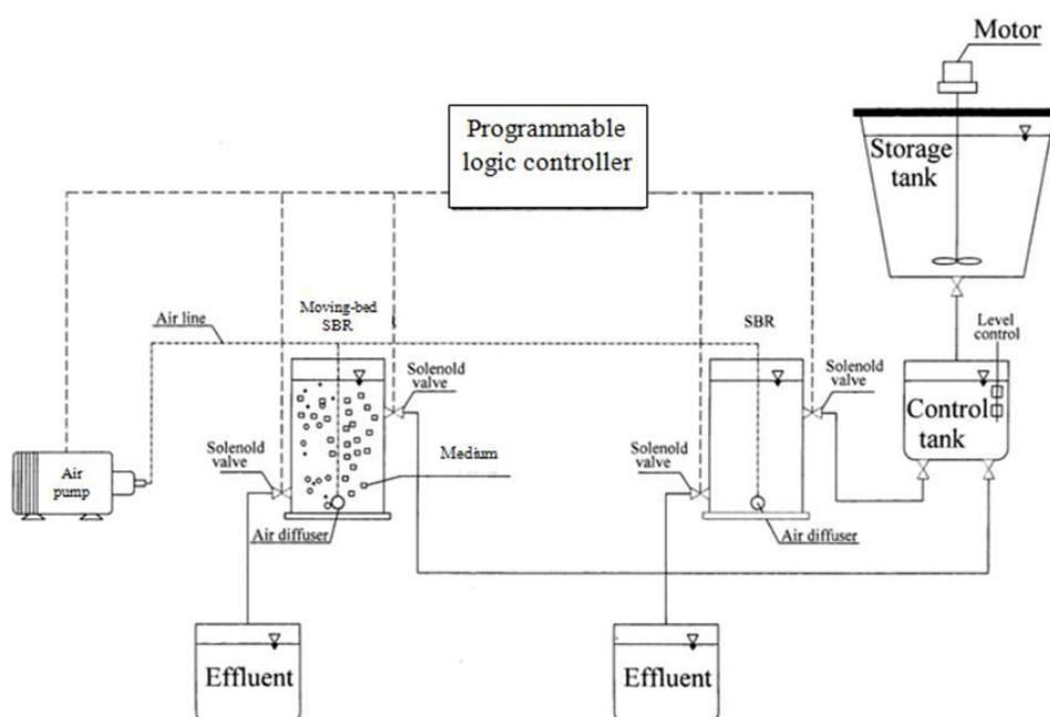
**Figure 1.** Schematic diagram of SBR and moving-bed SBR systems
