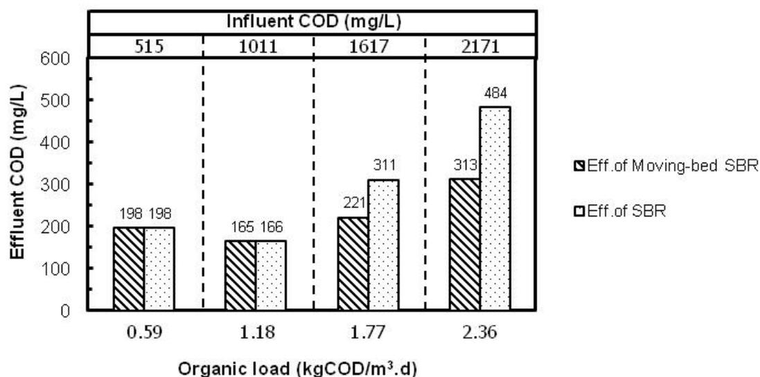
**Figure 2.** Relationship between effluent COD and organic load
