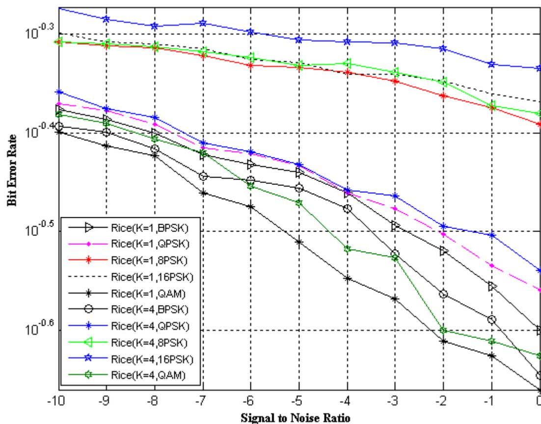
**Figure 4 (b).** A more comprehensive view of Figure 4(a) in which a variation is shown for lower values of SNR
