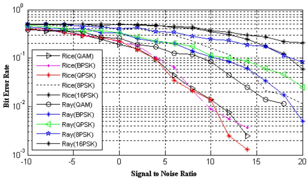
**Figure 3(a).** BER of concatenated STBC-LDPC scheme in Rayleigh and Rician fading with different modulation schemes
