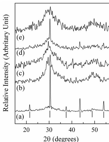
**Figure 1.** XRD patterns of the powders obtained from reactions between  $\text{ZrO}(\text{NO}_3)_2 \cdot \text{H}_2\text{O}$  and different lead precursors in  $14 \text{ moles dm}^{-3}$  KOH solution for 3 hours: (a)  $\text{Pb}(\text{NO}_3)_2$ , (b)  $\text{Pb}(\text{CH}_3\text{COO})_2$ , (c)  $\text{PbF}_2$ , (d)  $\text{PbCl}_2$  and (e)  $\text{PbI}_2$ . The vertical bars indicate diffraction characteristics of PZ (ICSD 077-0856).
