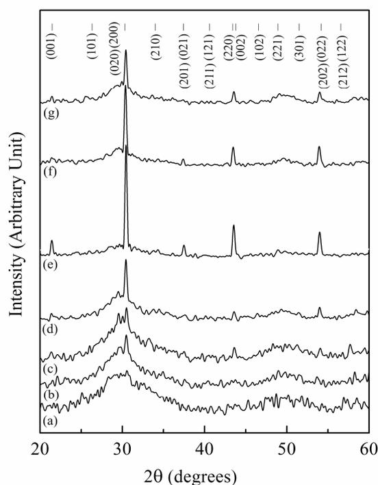
**Figure 2.** XRD patterns of the powders obtained from the reaction between  $\text{ZrO}(\text{NO}_3)_2 \cdot \text{H}_2\text{O}$  and  $\text{Pb}(\text{NO}_3)_2$  at 720 W for 3 hours in different concentrations of KOH solution: (a) 6 (b) 8 (c) 10 (d) 12 and (e) 14 moles  $\text{dm}^{-3}$ , compared to those obtained in 14 moles  $\text{dm}^{-3}$  KOH solution with different reaction times: (f) 4 hours and (g) 5 hours. The reference pattern is shown with vertical bars (ICSD 077-0856).
