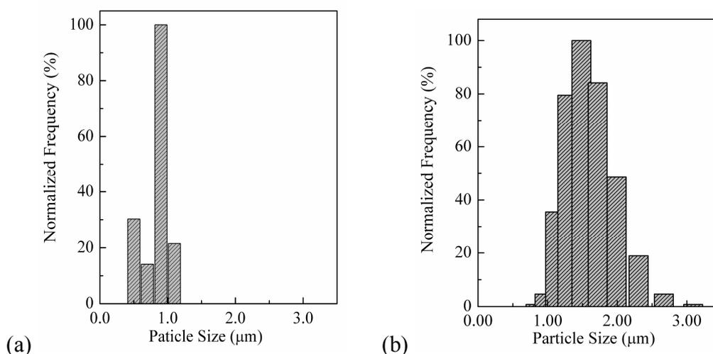
**Figure 4.** Particle size distribution of the cubic PZ particles measured from (a) FESEM images and (b) light scattering experiment (measured on the same powder sample)
