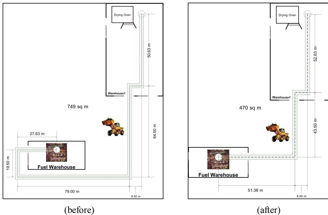
Figure 5. Layout modification of the transferring of firewood to the dryer
