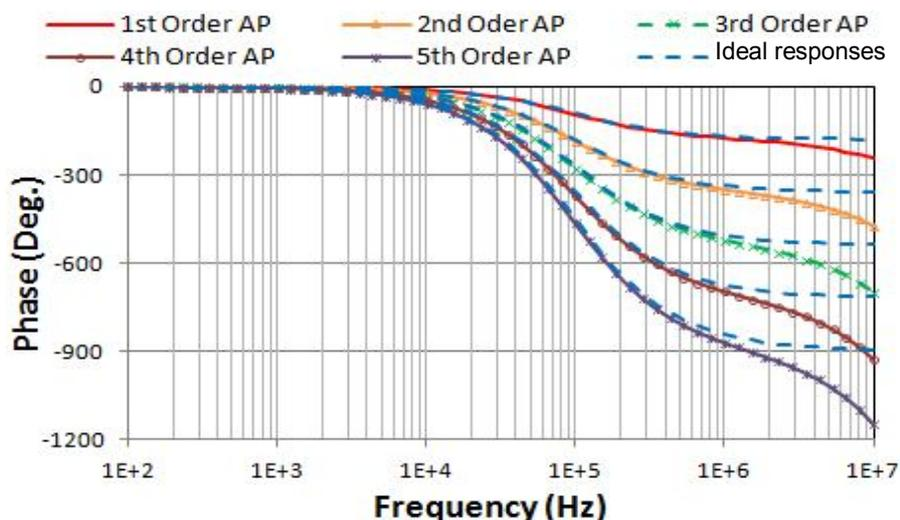
**Figure 7.** Simulated phase responses of higher-order AP filters
