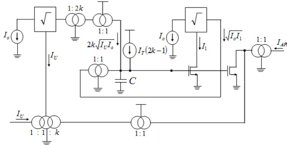
Figure 2. Proposed low-voltage SRD design of first-order AP filter
