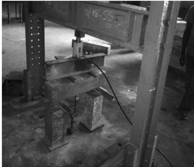
Figure 2. Testing arrangement of beam specimens
